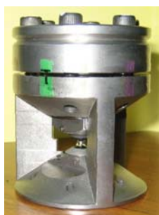
Fig. 2.4. A panoramic diamond anvil cell. Compared to symmetrical DACs, panoramic DACs have more side openings hence allowing detection of inelastic signals.
